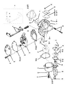
Figure 15 Carburettor assembly
