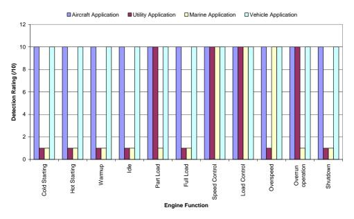
Figure 4 Detection Rating for engine functions and engine groups
