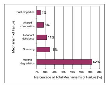
Figure 12 Percentage of total mechanism of function failure
