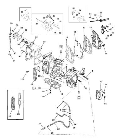
Figure 18 Cylinder block assembly
