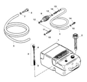
Figure 14 Fuel tank assembly
