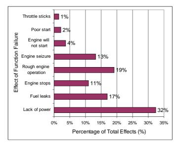
Figure 11 Effect of component function failure on engine operation
