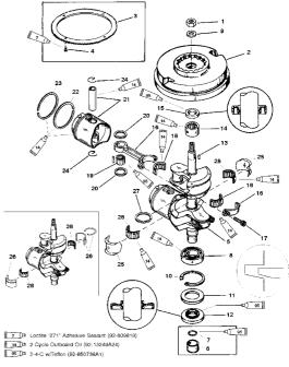
Figure 17 Crankshaft assembly
