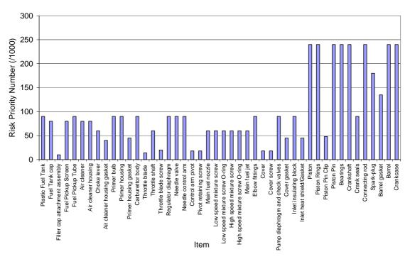
Figure 13 Risk Priority Number for components of FS45 Line-trimmer engine
