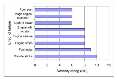
Figure 7 Severity rating of the effect of failure for components exposed to E20
